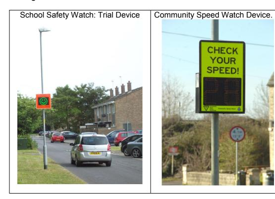
SSW devices cost approximately £2000 each. This is similar to the CSW signs. Both signs are powered by rechargeable batteries.
